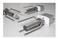
The impact sound insulated shear force dowel Egcopal reduces impact sound by decoupling components. It is used for the bedding of stair landings, arcades and cantilever balconies and transmits the shear forces acting in the connection joint. At the same time, the acoustically decoupled bedding ensures that the transmission of disturbing noises into adjacent rooms is insulated
